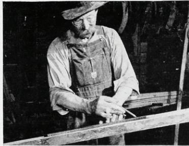
UNCLE ALEX USES A WOOD TEMPLET to mark out rim sections on a piece of white oak timber. Others hang in row in back of him.
