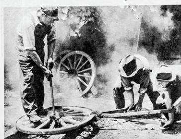
With long pincers, a nearly red-hot tire is clamped onto a wheel.
