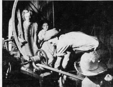
BENDING A WAGON TIRE INTO SHAPE. Tires come in long flat bars of steel and are fed through hand turned roller to fit the wheel.
