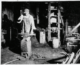
WADE CLINE CAULKING HORSE-SHOES. The shoe must be caulked and fitted to each foot individually—by the skilled blacksmith.
