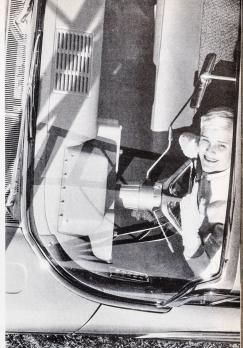
BIGGEST WINDSHIELD of all is Mercury's. As shown here from it slopes up, almost over driver's head, and also comes far around to the side.
