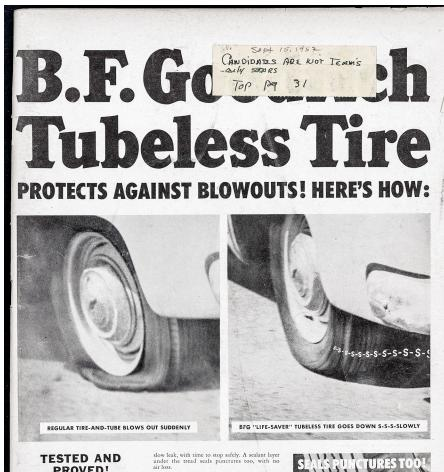
Most blowouts start when you don't know it, from a share blow-for instance against a curbo chuckhole-that bruises cords inside the tire. As the tire flexes, the weak spot grows und it in ner wall is broken. With a regular tire and tube months later, the tube is pinched and blows out through the tree.
