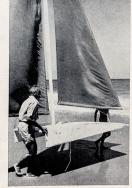
LAUNCHING the plywood boat, Lowell Christ-man and Heidi easily lift it and carry it bow first to-ward the surf. Projecting down from the sides of the hull are two thin, tapered fins which act as keels.
