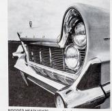
HOODED HEADLIGHTS, wrapped by the sweeping fenders, are a feature of Lincoln, which also has parking lights in humper.
