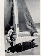
LAUNCHING the plywood boat, Lowell Christman and Heidi easily lift it and carry it bow first toward the surf. Projecting down from the sides of the hull are two thin, tapered fins which act as keels.
