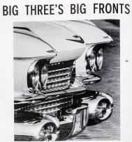
MASSIVE GRILLE of Cadillac is honeycombed, has recessed lights in bumper, headlights set between grille guard and fenders.
