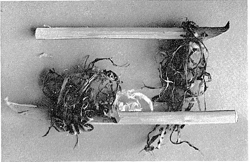
FIGURE 3. Planer knife shavings. Square ends were cut with an abrading knife.
