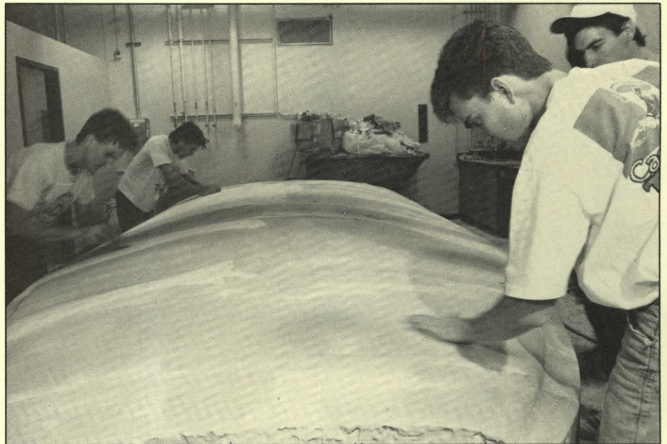
Engineering students work on the plaster mold from which the solar car's hull will be cast.
