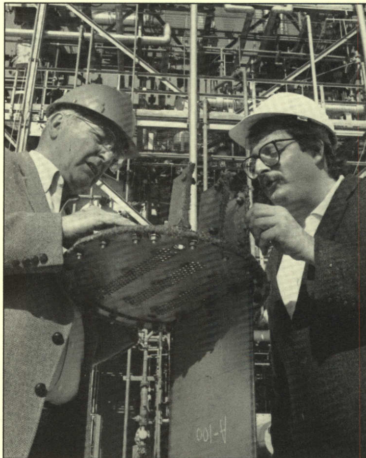
Center researchers are testing distillation components invented by Trent (left) and Byron Parker of Salt Lake City, Utah. Jose Luis Bravo (right), manager of the Separations Research Program, said the testing, done in the center's pilot-scale distillation tower, is sponsored by the US Department of Energy and the National Bureau of Standards.
