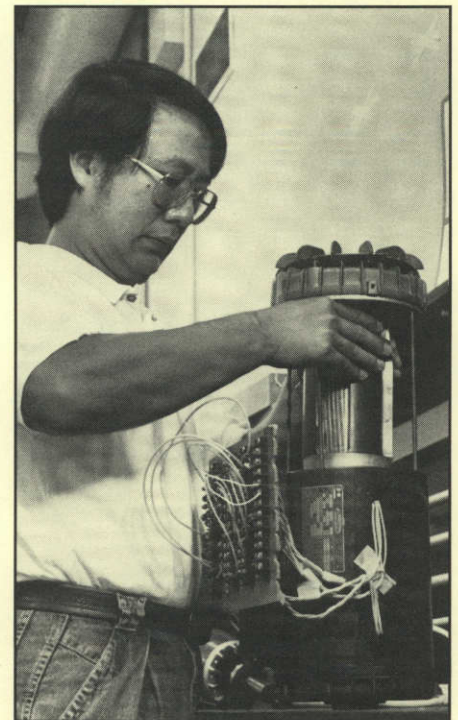
Researcher Shy-Shenq Liou places a rotor inside a prototype reluctance motor. In testing, the new motor showed approximately double the normal torque capacity.
