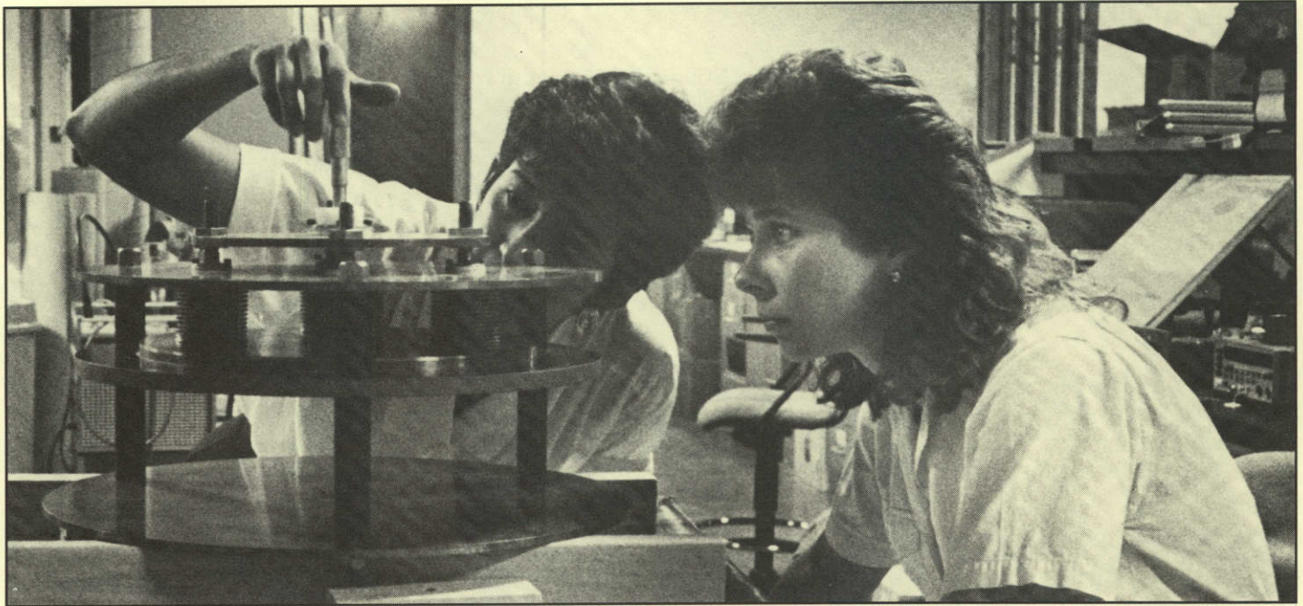
Engineering graduate students Anita Ortiz (left) and Jill Bailey-Duckworth measure the dielectric properties of gypsum board.
