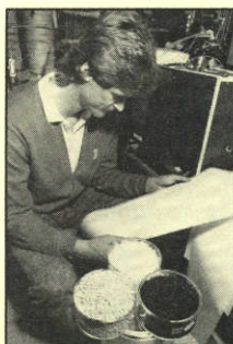
Finnish researcher Harri Järvelin and others are separating propane from propylene with adsorption under low pressure.
