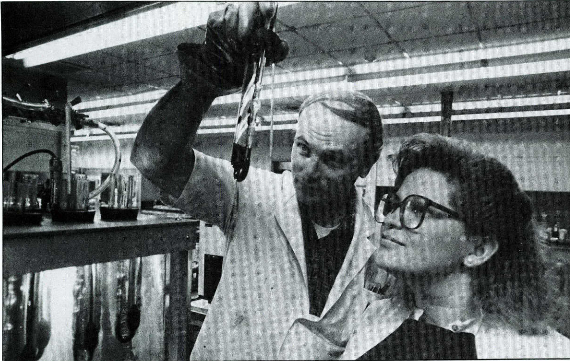
Technicians Larry Miller and Cathy Teinert observe the results of an asphalt viscosity test.
