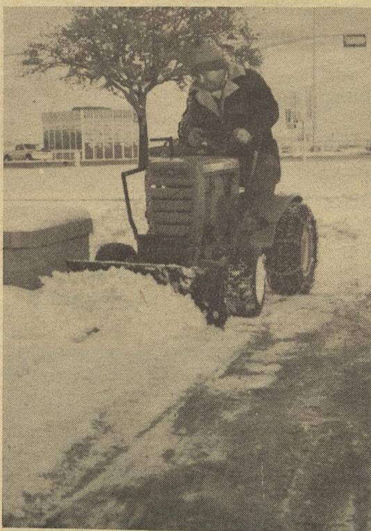
District 7 employees converted a yard tractor to a "mini-snowplow." (Photo by Gene Hirschfelt)
