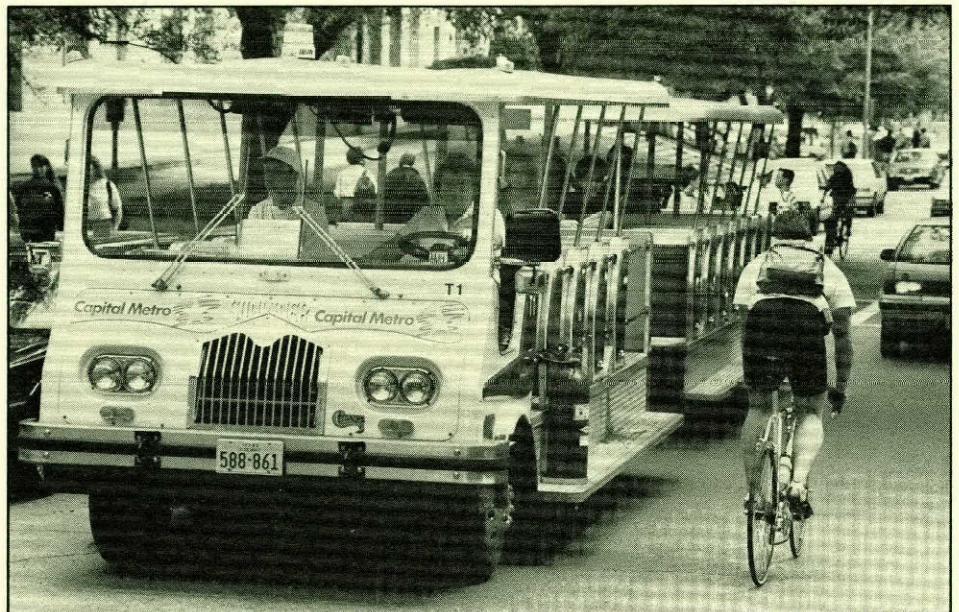
UT Austin and Capital Metro are running an eight-week experiment with a free open-air tram powered by propane. The shuttle, METRAM, a red-and-white 48-seat trolley, has proven popular among students in its first weeks of operation in March on the UT Austin campus.
