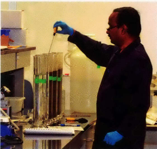
Chemist K.M. Rahman takes hydrometric measurements of sand, silt, clay, and gravel in a sediment sample.
