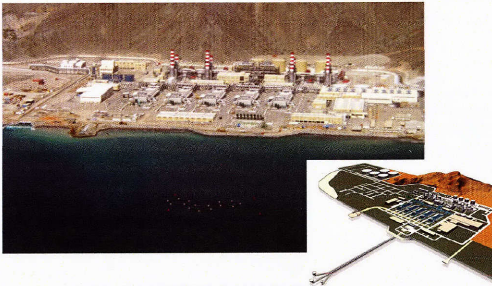
Figure 9-4: Off-shore Open Intake
