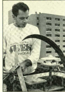
Mechanical engineering graduate student Chrys Hadjimarkos checks a shadow-band pyranometer on the roof of the Engineering Teaching Center.
