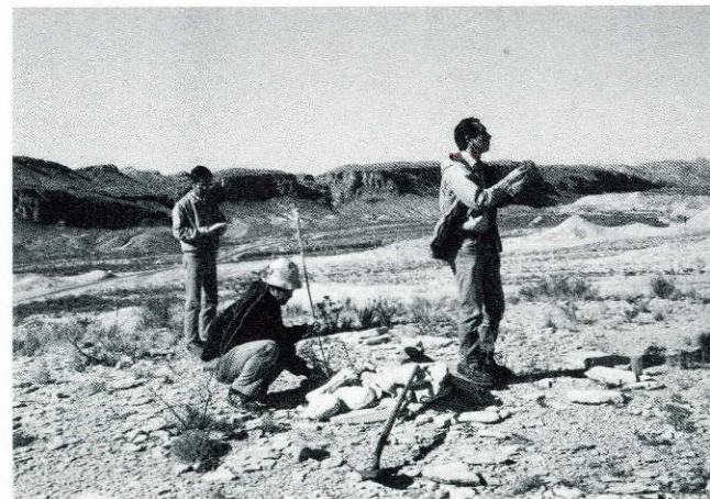
Roberto Gutierrez (right) measures the elevation of the horizon at the location of a National Geodetic Survey benchmark (near Terlingua, Texas) being inspected by fellow graduate student Young Sun Nam (center) while faculty member Yosio Nakamura looks on. This location was examined as a possible site for a Global Positioning System survey point to measure tectonic motion in West Texas.
