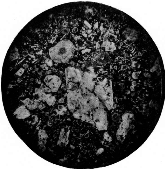
Figure B. Micro-photograph of a thin section of altered igneous rock taken from Well 73, Thrall Oil Field, showing the structure of the original basalt. Plane polarized light. Magnified about forty diameters. Photograph by W. H. Tomlinson. Compare this rock with that shown in Plate VII.
