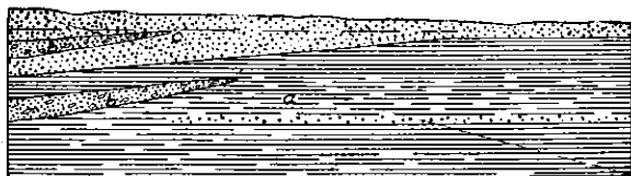
FIG. 2. Wichita beds exposed in the bank of a creek in T. T. Railway Company survey, 9 miles north and 2 miles west of Iowa Park, Wichita County: a, shale; b, conglomerate; c, sandstone.
