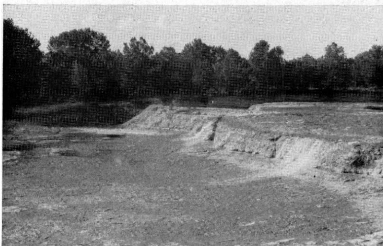
Figure 15.—Chalky and marly beds of the Austin formation exposed in the spillway of White Rock Reservoir.
