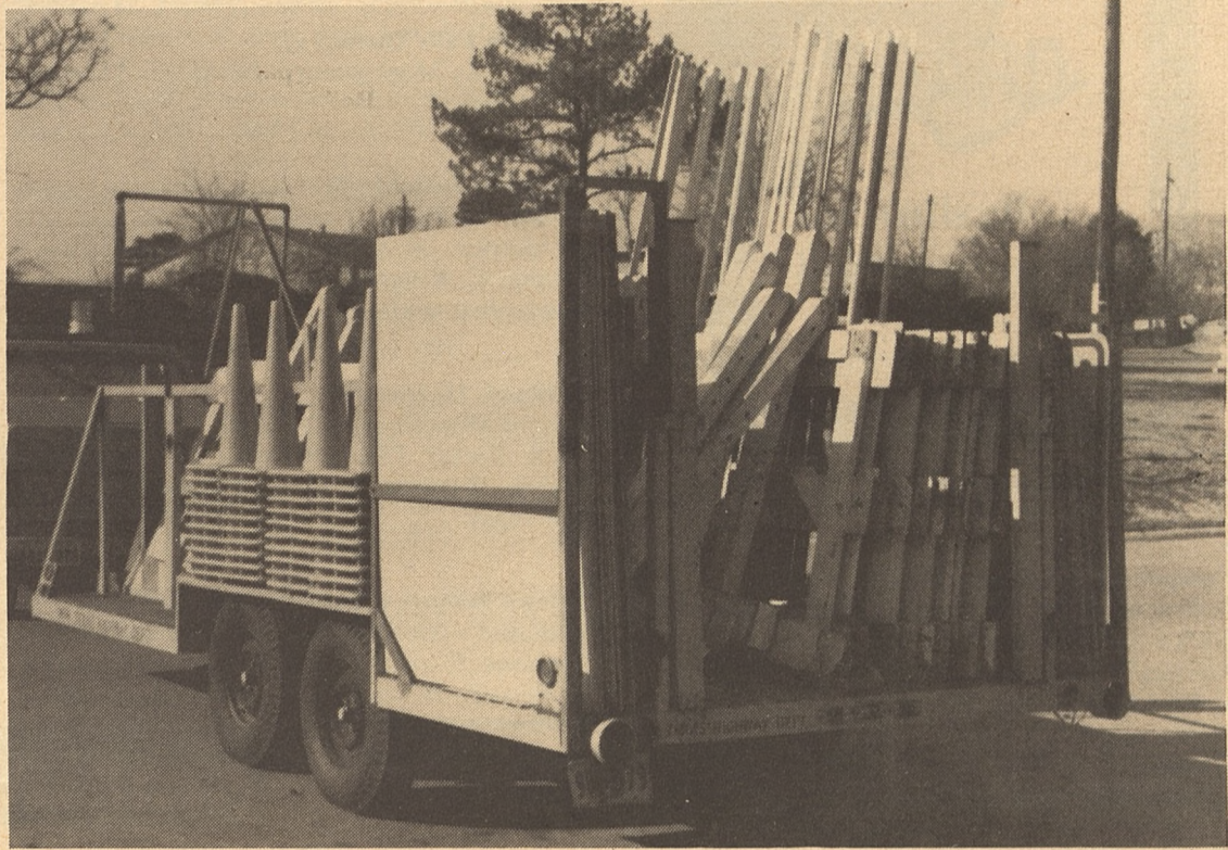
Organization and efficiency dictate the arrangement of traffic control devices on Longview's loaded sign truck. (Photo by Laura Rayburn-White)
