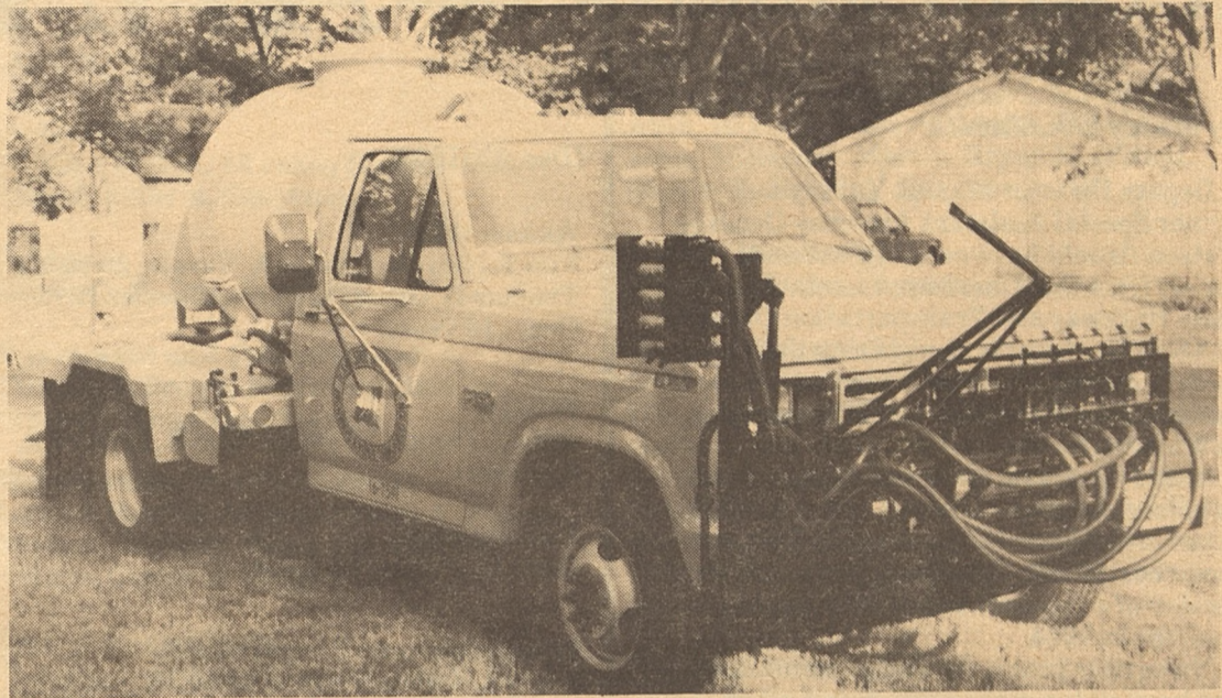
Herbicide trucks featuring "Flex Five" system of sprayers, built by Equipment and Procurement Division shops, give operators fingertip control. (Photo by Bob Gates)
