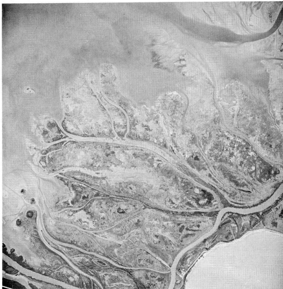
FIG. 2. The Trinity River delta. River deltas have variable shapes, depending upon the local environment. Some of the controlling factors are: volume and velocity of water and the number of stream tributaries, the character of the water basin, strength of ocean currents, prevailing wind direction, and presence of offshore bars or other shoreline features. (Photograph by U. S. Department of Agriculture, Salt Lake City, Utah.)
