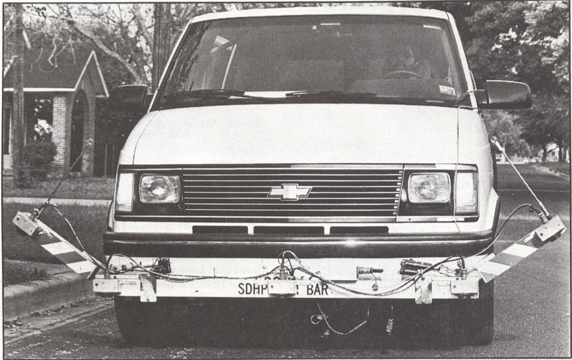
Van equipped with ultrasonic sensors uses sonar to measure rutting in asphaltic pavement. Old-fashioned yet fairly reliable "rutometer," right, uses string, stick to detect rutting. (Photos by Gay Shackelford, Travel and Information Division)
