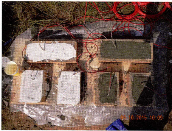
(c) Curing compound application
