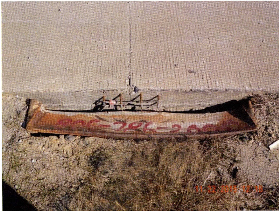
Figure 4.12 Destroyed gages during the FDR on SH 288
