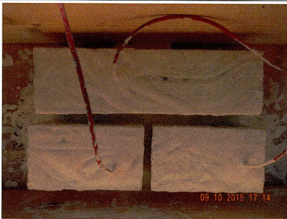
(d) Fully coated prism with curing compound
