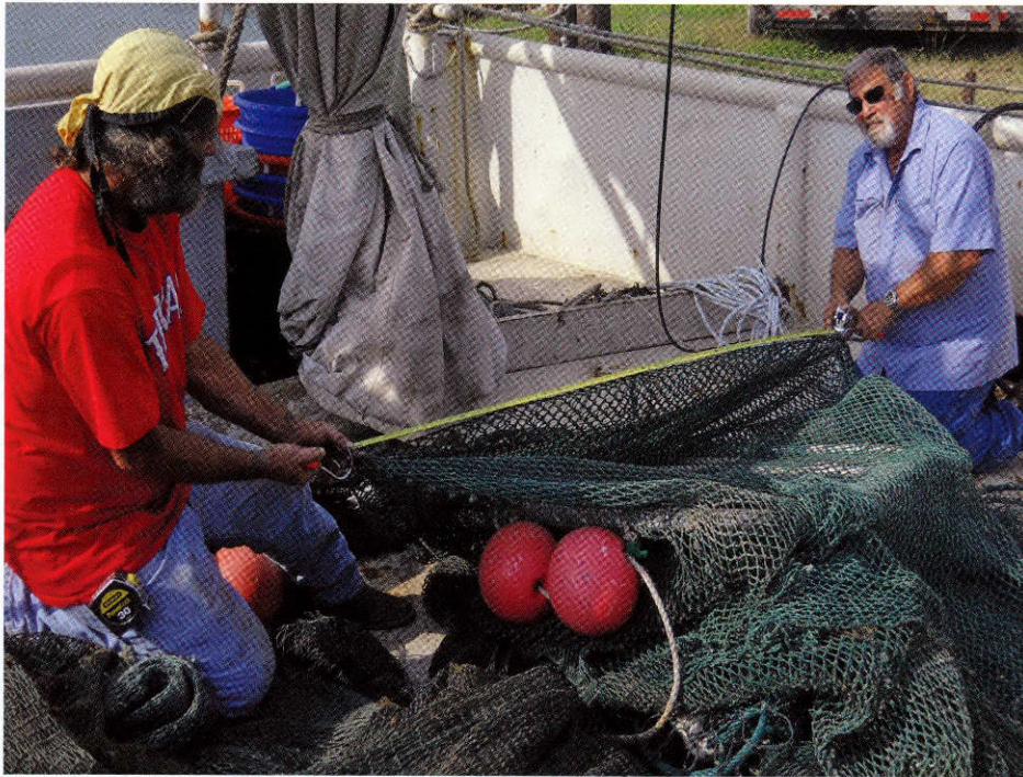
Graham helps a shrimp fisherman in Port O'Connor check his turtle excluder device.
