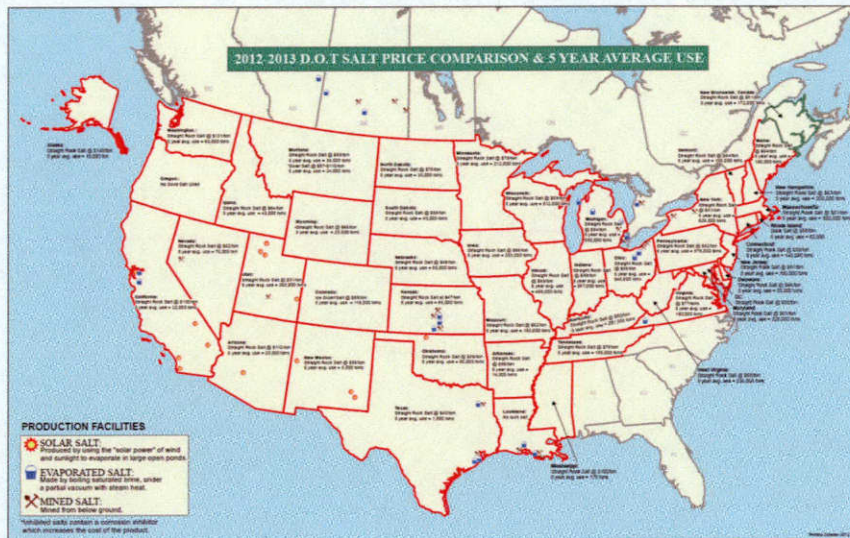
FIG 21. Salt Sources, Cost Comparison and Usage Based on 2012-2013 State Survey (source: Washington State DOT).
