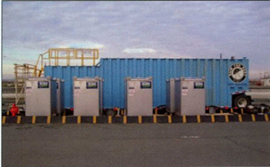
FIG 35. TxDOT districts south of IH20 should use pre-blended brine with temporary storage in frac tanks
