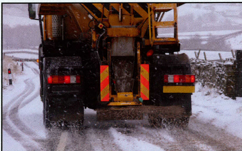
FIG 38. Calibrate granular material spreaders so that the material applied corresponds to the target application rate
