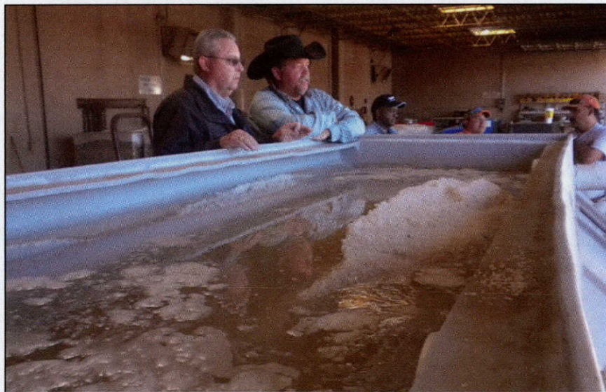
FIG 34. In-house salt brine manufacturing units with permanent on-site storage tanks are used in the northern snowy districts
