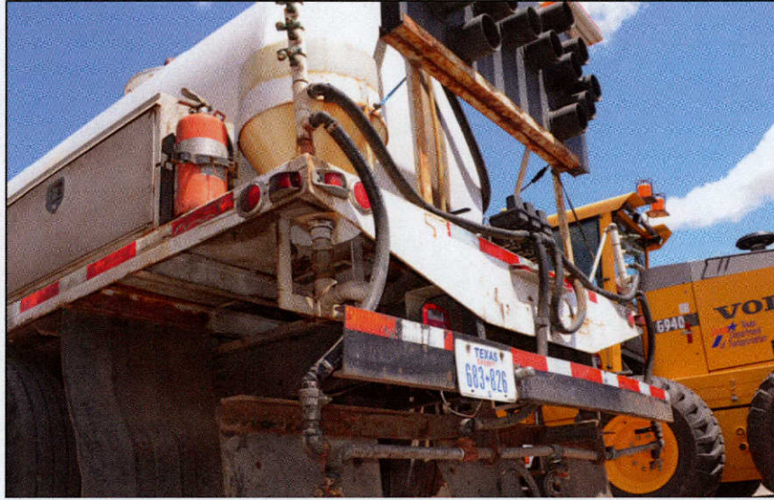
FIG 39. Thoroughly and completely power wash snow and ice application equipment after storm events
