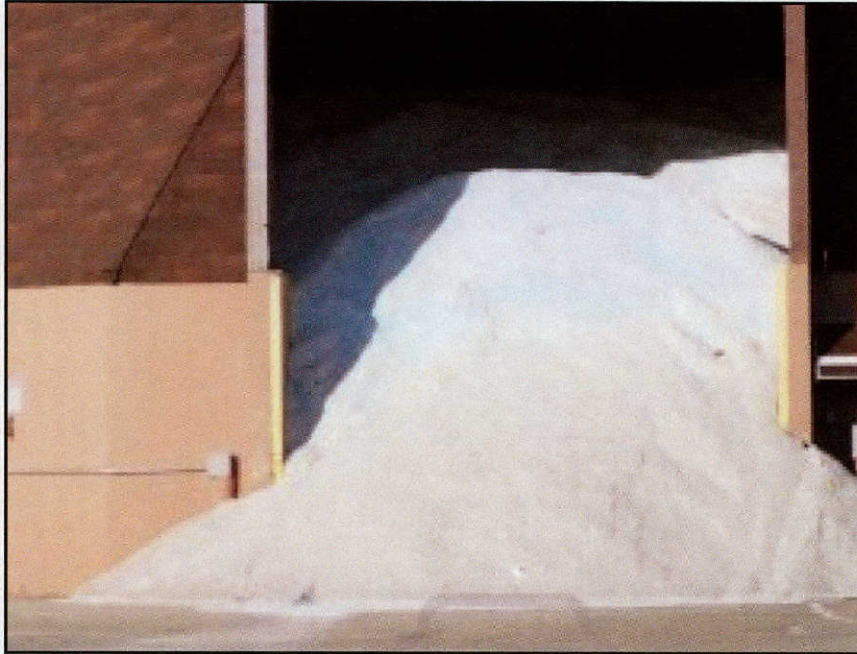
FIG 15. Road salt (NaCl) for maintenance applications is the granular form of sodium chloride
