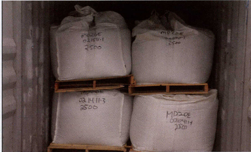
FIG 33. For TxDOT districts south of IH20, storage of granular material in 2500 lb super-sacks is recommended
