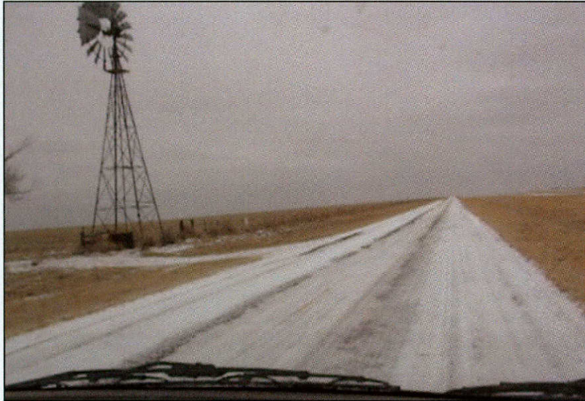
FIG. 20. Road Surface Condition Before Plowing, Drive Lane Treated w/Road Salt for De-Icing/ Opposite Lane Not Treated (Control)
