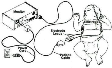
This picture shows the correct way to connect the infant to the MONITOR. The ELECTRODE LEADS are plugged into the PATIENT CABLE which in turn connects to the MONITOR. The MONITOR is connected to the wall socket by the POWER CORD.
