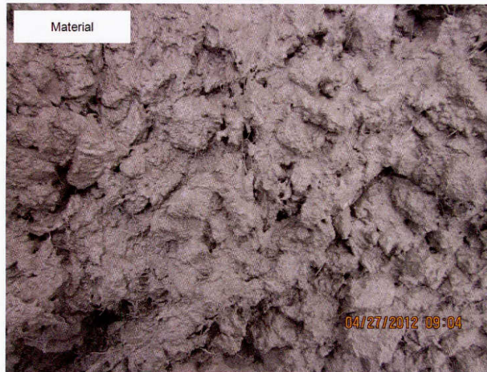
Figure 3.9 Fiber in Concrete
