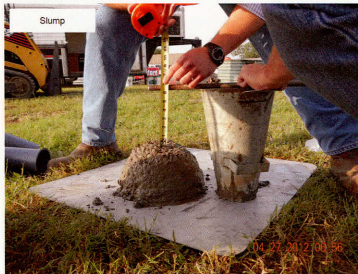
Figure 3.8 Concrete Slump Test
