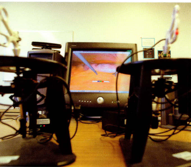
Behind the haptic devices that allow for the virtual sensation of touch is the computer screen showing virtual surgical instruments that are controlled by the mechanical haptic devices.
