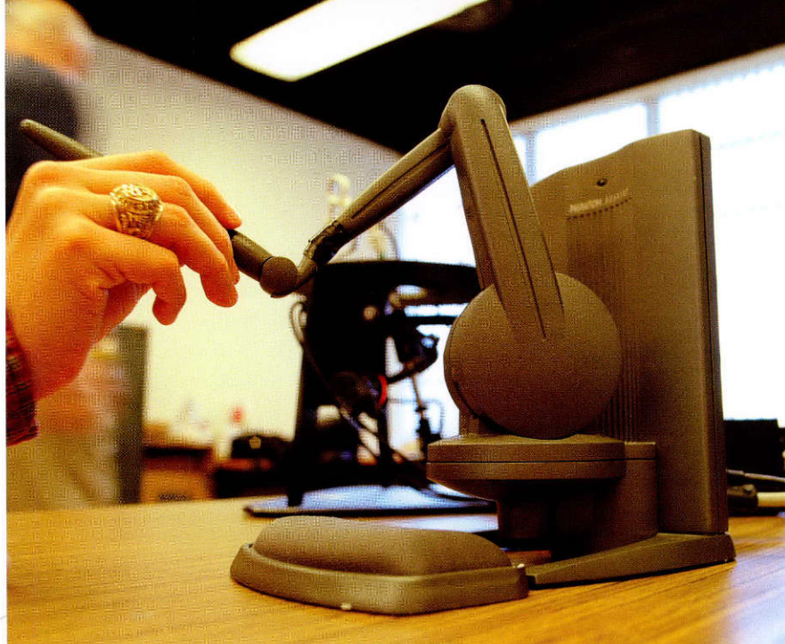
This haptic device allows users to reach into a virtual patient to clamp and snip blood vessels through the virtual sensation of touch in three-dimensional form.
