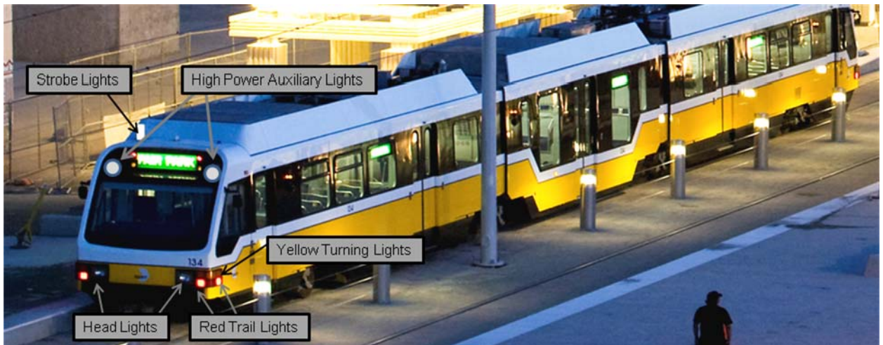
Figure 48: DART Rail Vehicle Night Lighting
