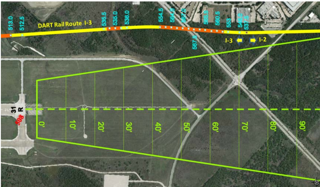
Figure 13: Runway 31R, Part 77 Approach Surface
