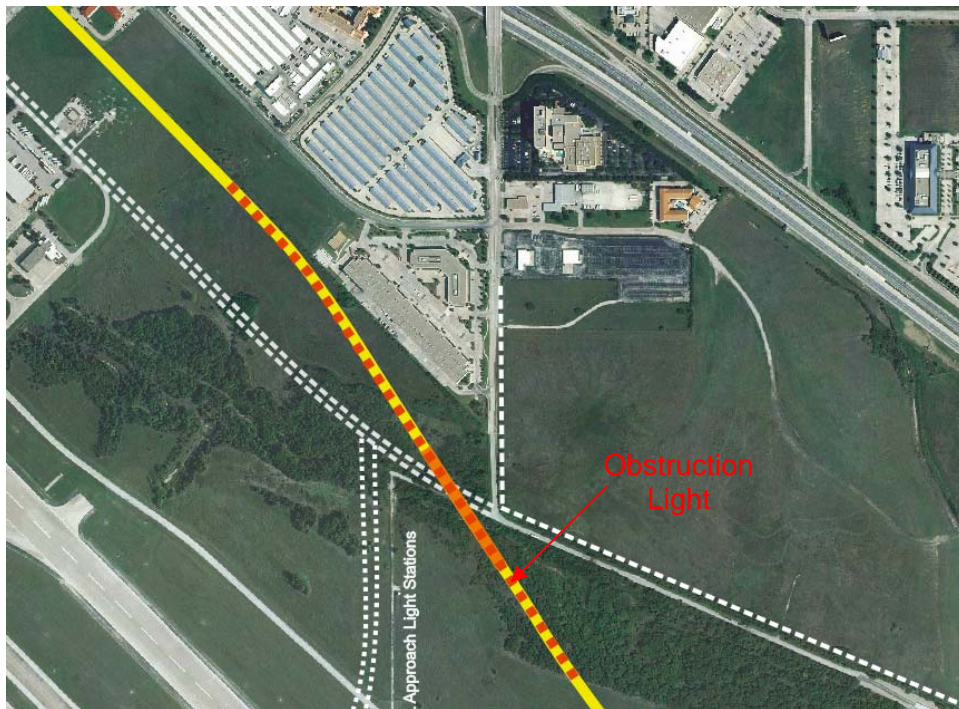
Figure 2 Catenary Pole Obstruction Lighting Area Runway 17L
