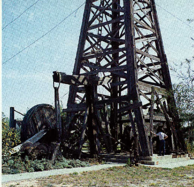
Vintage cable-tool drilling rig, Pioneer Park in Kermit
