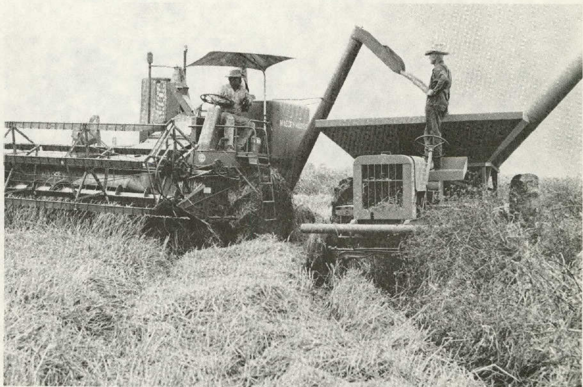
Harvesting irrigated rice near Beaumont. Grain is being transferred from combine to "double bug" for transport out of the field. Photo courtesy U.S. Soil Conservation Service.
