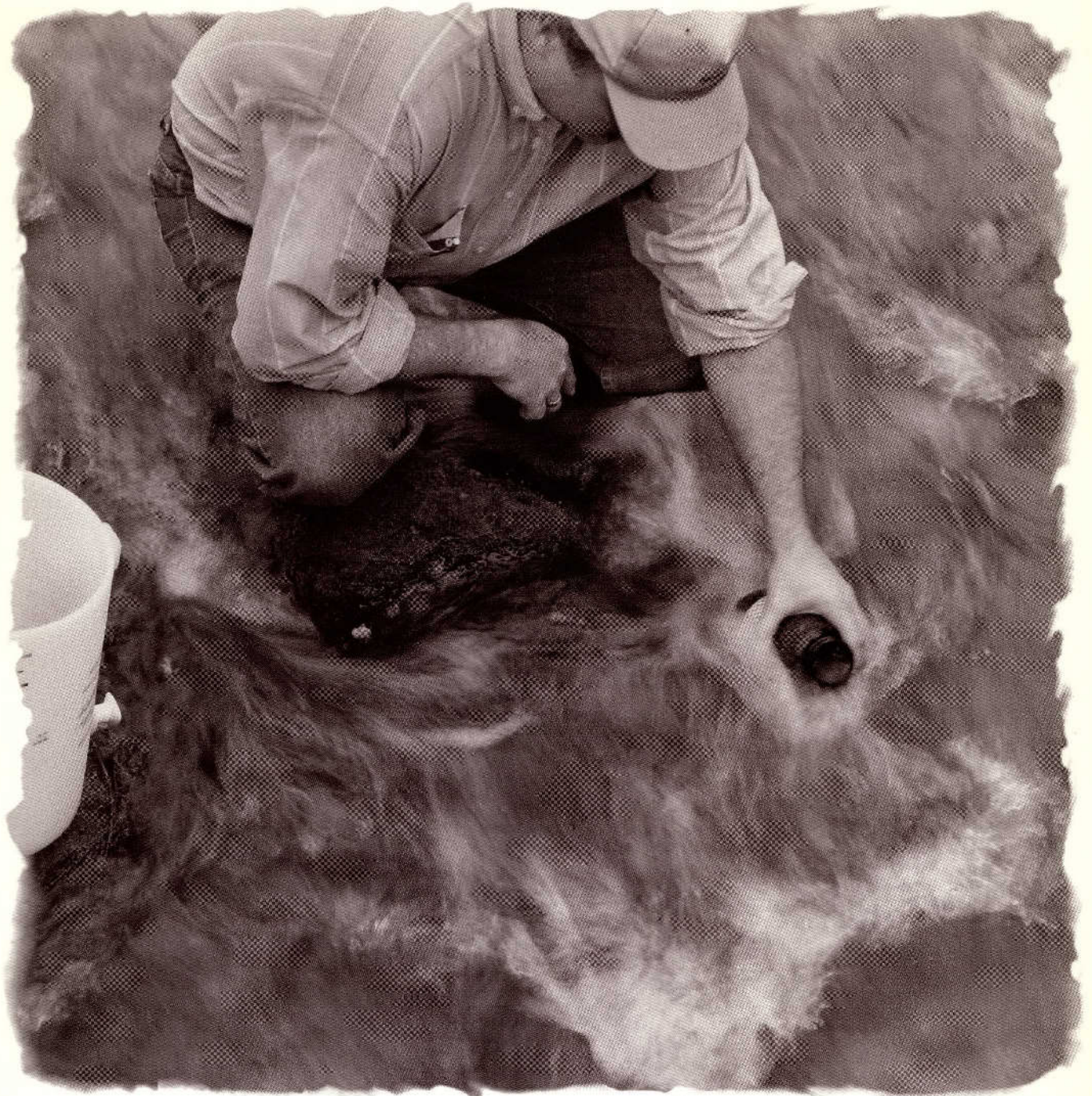
Hydrologist John Waugh samples surface water near Hueco Springs in Comal County. Samples are taken throughout the Edwards Aquifer region on an annual basis to monitor the water's quality. The samples are analyzed for pesticides, herbicides, metals, volatile organic compounds and other parameters that could contaminate the excellent quality of aquifer water.
