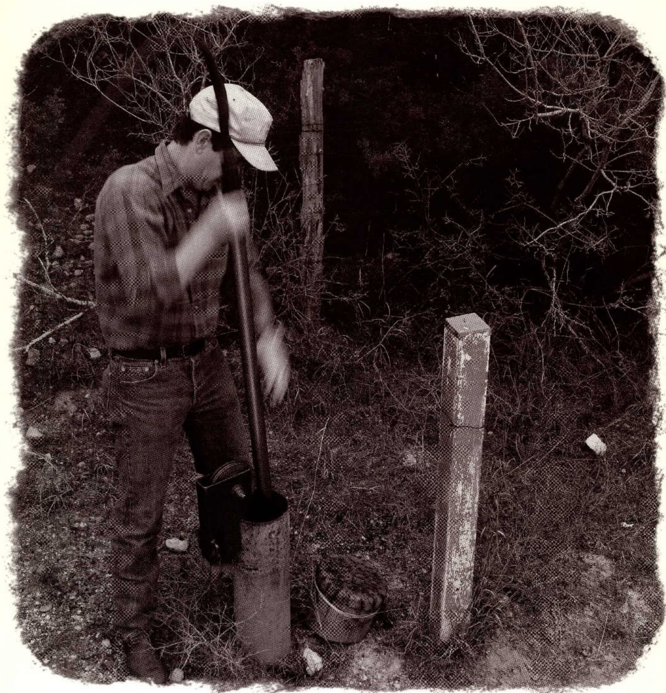
Hydrologist Jim O'Connor lowers a geophysical logging tool into a well bore. The tool is used to measure the thickness of and the depth to different rock or clay formations. This well is located on the recharge zone. Here, the Edwards Aquifer is 432 feet below land surface.
