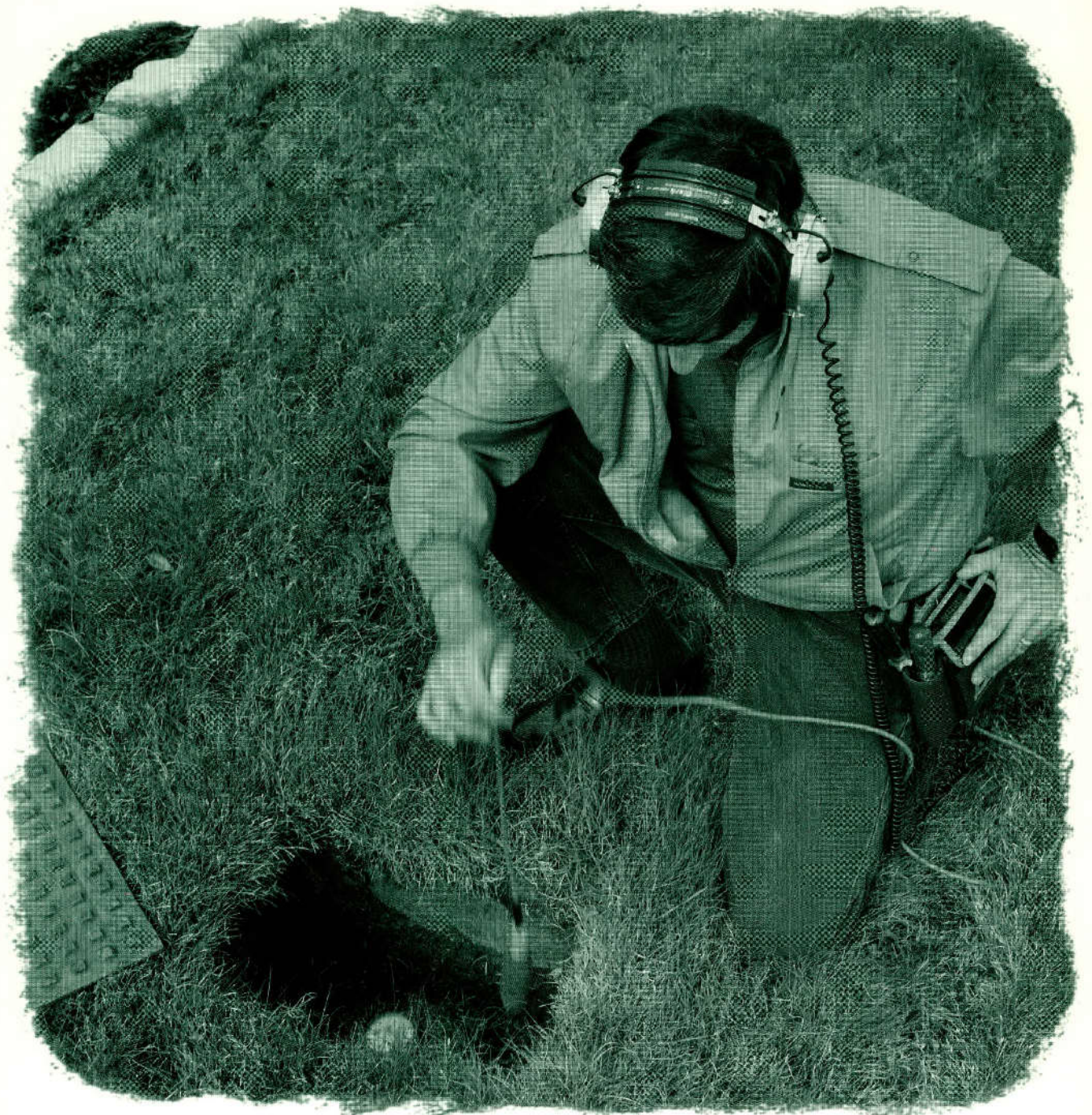
Leak Detection Technician Jim Shipley listens to a water meter. He is using equipment which electronically amplifies the acoustical signal created by pressurized fluid escaping from a pipe or valve.
