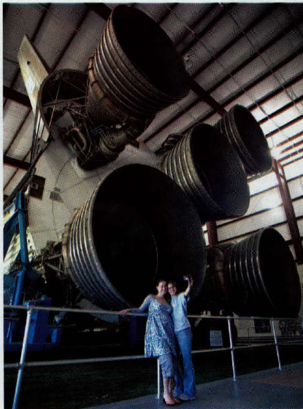
Blast off! The Saturn V's five engines, fueled by liquid oxygen, liquid hydrogen, and kerosene, together produced 7.5 million pounds of thrust.
