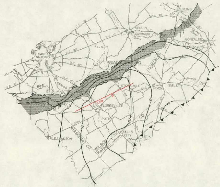
Proposed Line of Wells (Line A) Pumping 20,000 Acre-Feet Per Year Under Water - Table Conditions
