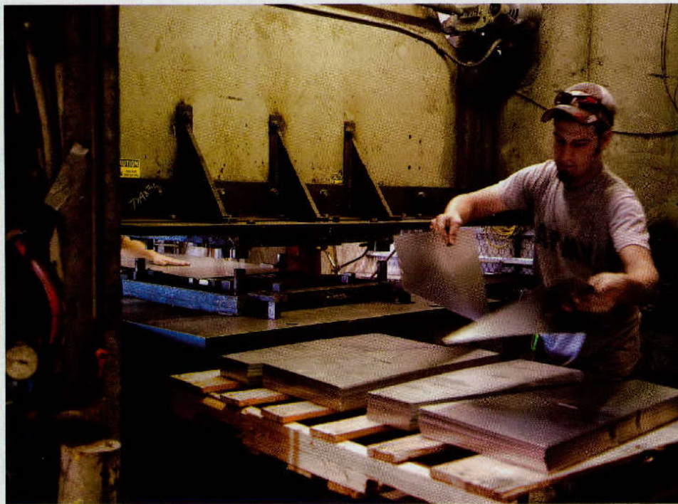
Justin Herman cuts sheet metal into sails at the Aermotor Company in San Angelo. Most Aermotor components are manufactured at this location.
