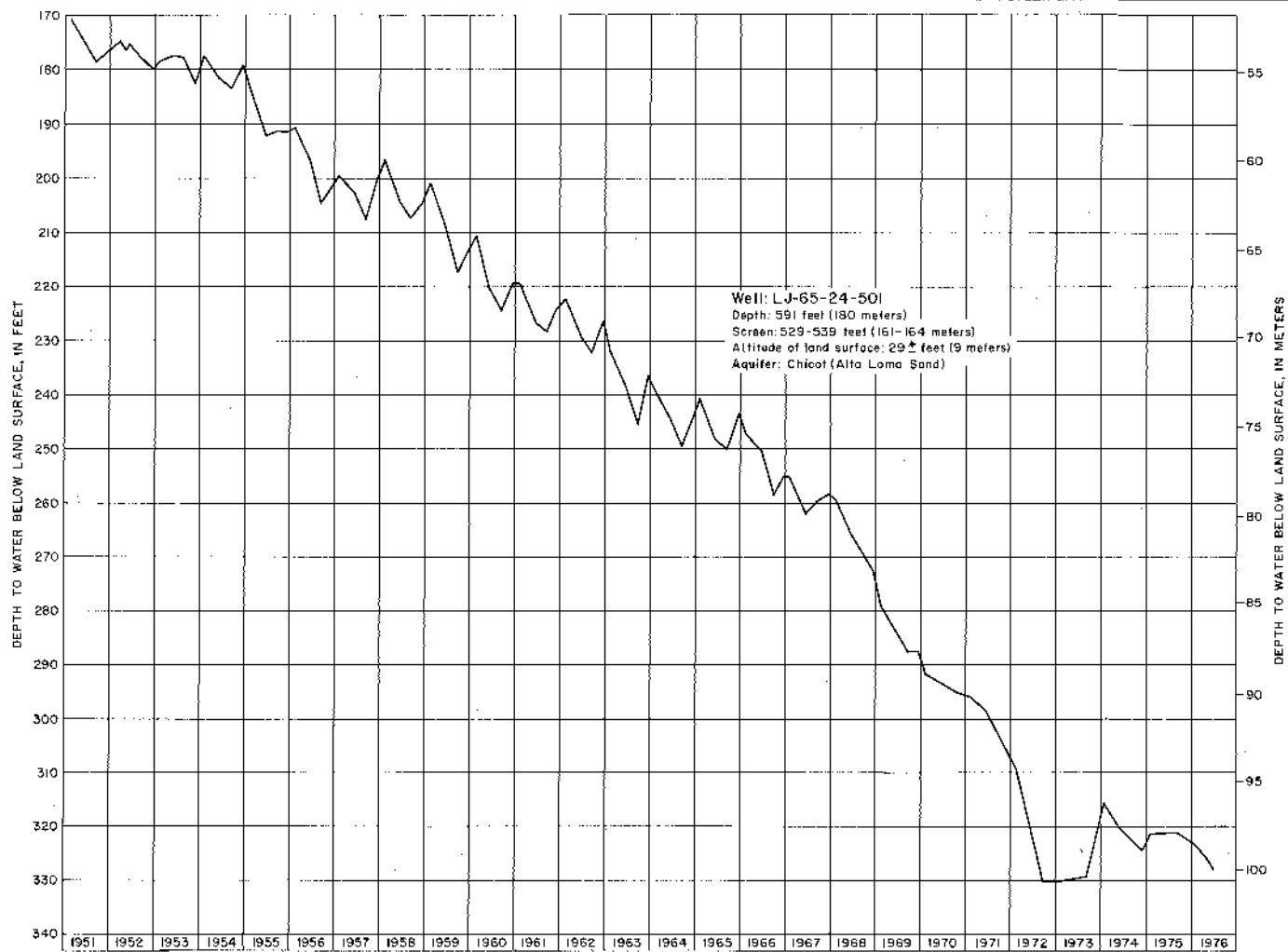
Figure 14 Hydrograph Showing Changes in Water Levels in a Well Completed in the Alta Loma Sand in the Baytown-LaPorte Area
