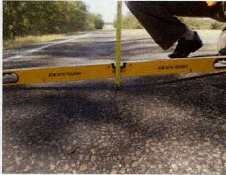
Figure 4.1 Measurements of rutting in the FM2 pavement
