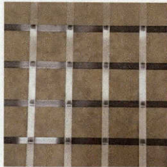
Figure 3.4 Baseline biaxial laser-bonded geogrid from polypropylene: GG 4
