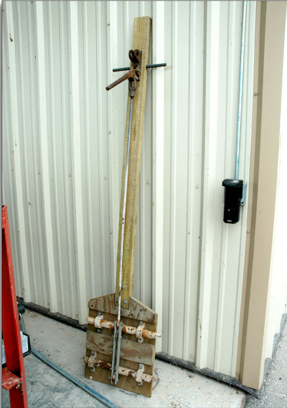
Figure 202: Wooden turn-out gate (rot gate), constructed by Cameron County Irrigation District No. 2 in 2007.
