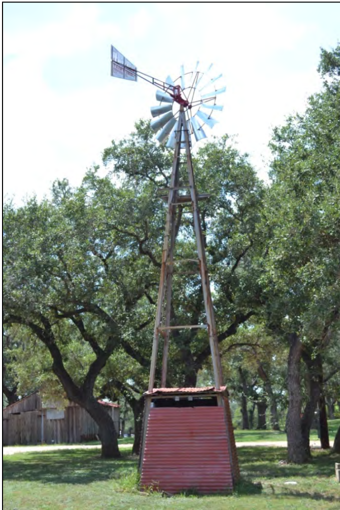
Figure 5-18. This metal windmill also has a metal-sided well house at its base.
