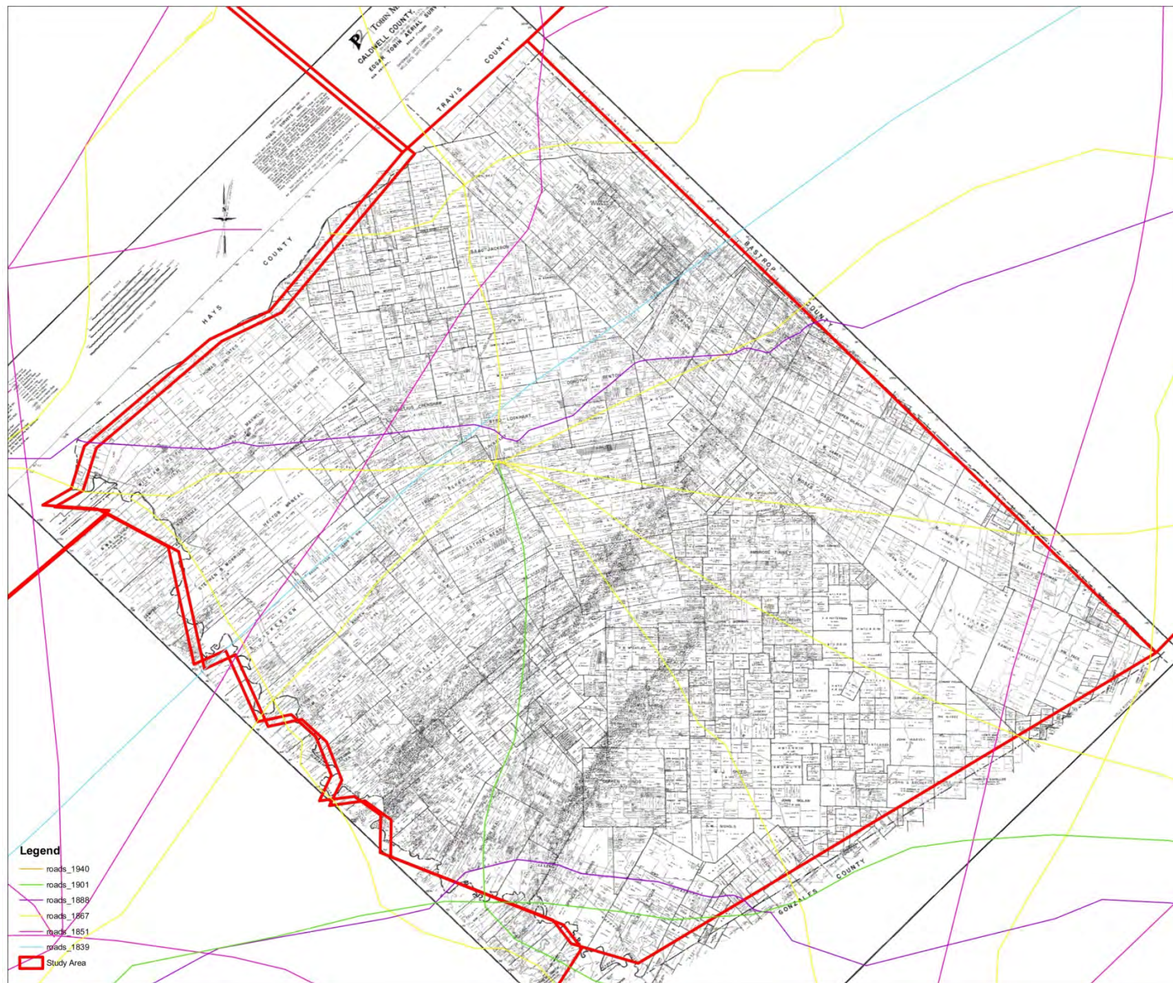
Figure 8-22. Evolution of Major Roadways and Road Network in Caldwell County Relative to Land Parcels. The map includes a Tobin map as the background, showing land ownership. The lines traversing the county represent roads that developed at different periods of time, their colors indicating their dates of construction. This “historic roads” shape file resulted from tracing road networks depicted on various historic maps included in the THO Collection. The objective in creating this map was to illustrate the development of road networks in Caldwell County over time and understand how the roads relate to the original land grants. Although the alignment of the roads does not appear to be precise in the overlay due to unavoidable geo-referencing issues, one can discern how the road networks were shaped by the land parcels.
