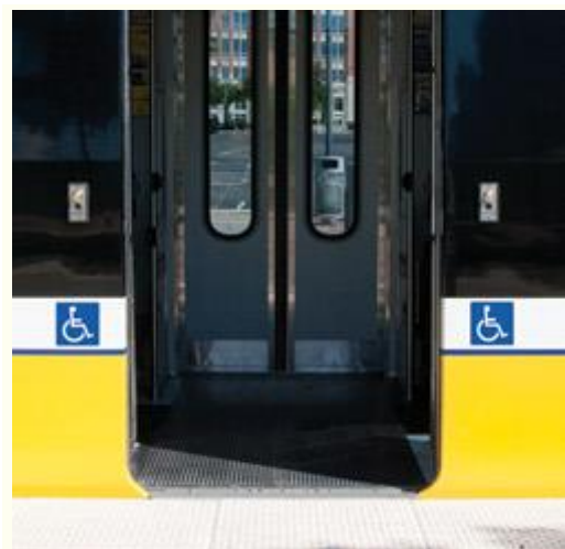
Low-floor doors open flush with the station platform.
