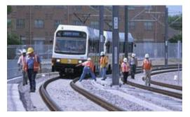
The tests are evaluating the operation of the new light rail track along the corridor. The first tests will determine if the right amount of electricity is getting to the vehicle as it travels the corridor. Electricity is transmitted to the vehicle through an overhead catenary wire from two electrical substations along the corridor.
