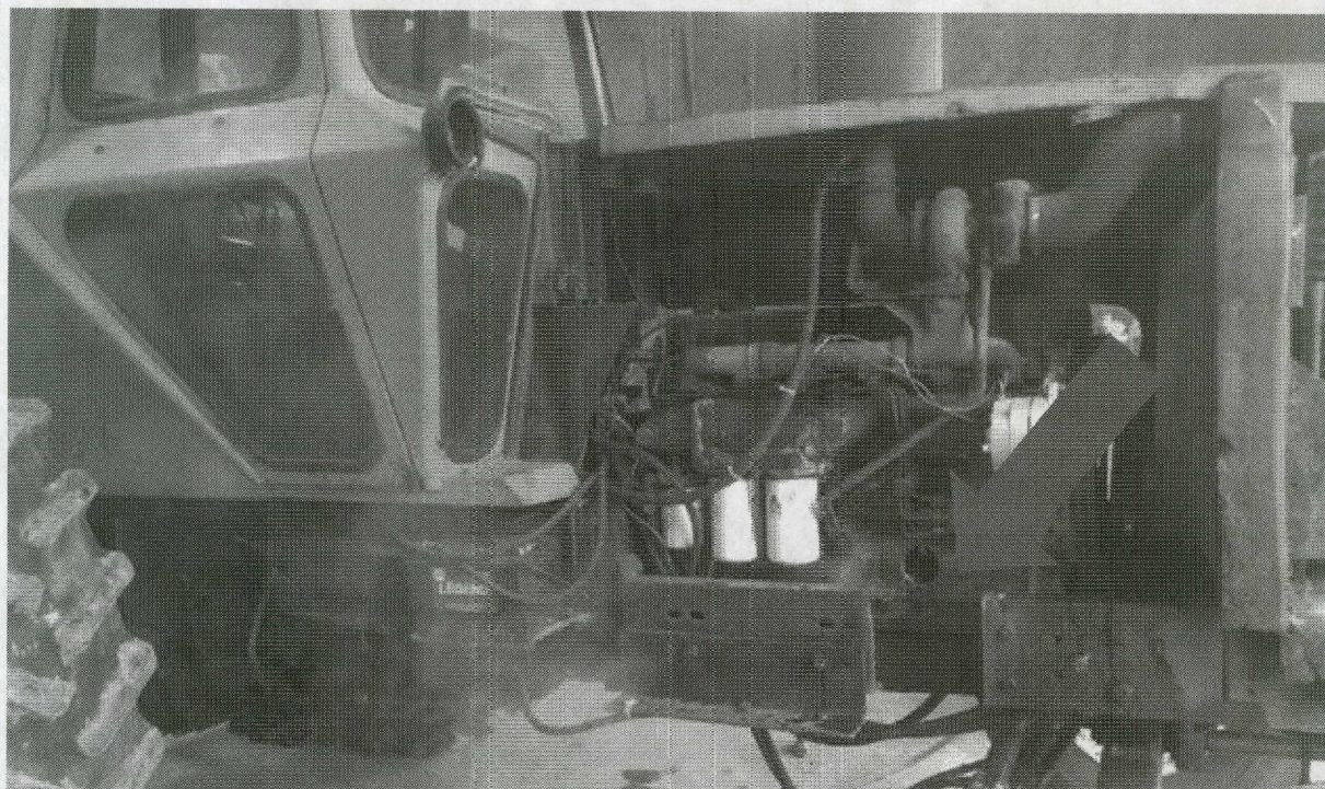
Figure 11. After Photo, with Frame Rail Cut
