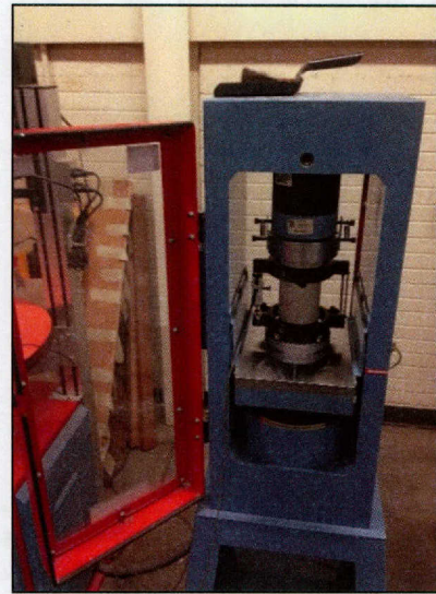
(b) Match-cured cylinder being tested
