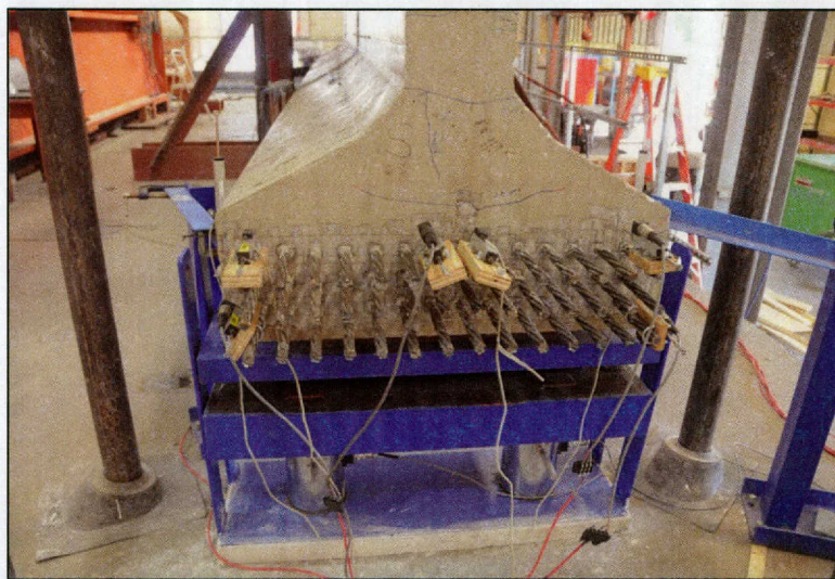
Figure 5-19- Displacement transducers used for measuring strand slip
