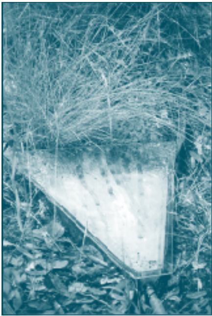
Each landscaping method was duplicated in a microlandscape. A triangular container captured runoff for analysis.
