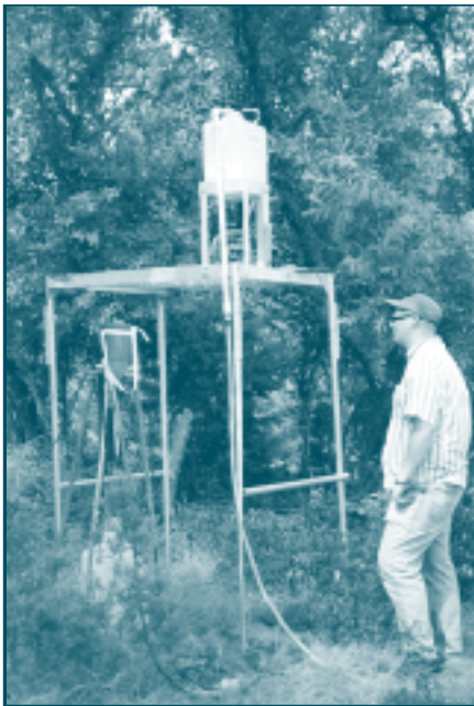
A rainfall simulator was used to measure the amount and type of runoff in each of the landscaping methods evaluated.
