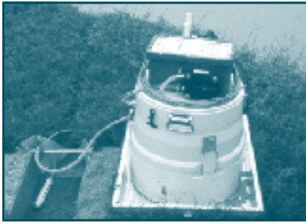
Automatic samplers were used to measure runoff.
