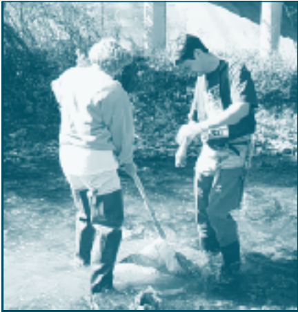
Texas Watch volunteer monitors learn a variety of chemical and biological monitoring techniques. Here, a volunteer learns how to use a kicknet. Volunteer monitoring raises local awareness and activism about water quality issues.
