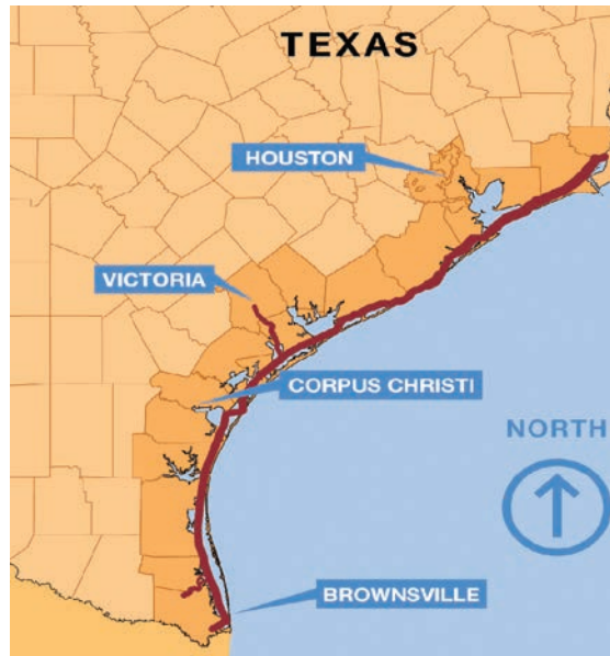
The GIWW is the nation's third-busiest inland waterway, with the 379-mile portion in Texas handling nearly 72 percent of its traffic (more than 80 million short tons in 2016). The GIWW in its entirety is classified as Marine Highway M-10 and the Texas portion is classified as M-69.
