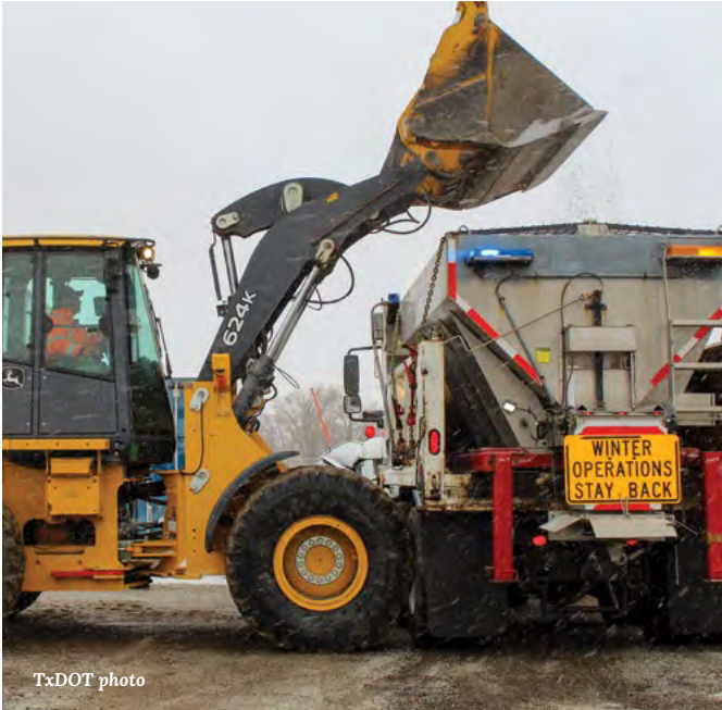
Lubbock District crews load salt onto trucks to prepare the roads for icy conditions.
