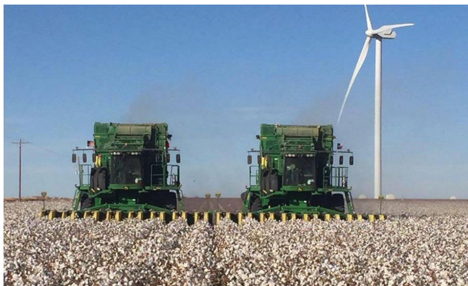
Cotton harvest in 2018. Dan said just one person can operate a John Deere CS690 cotton stripper-baler, replacing what used to be an entire crew. Courtesy photo.
