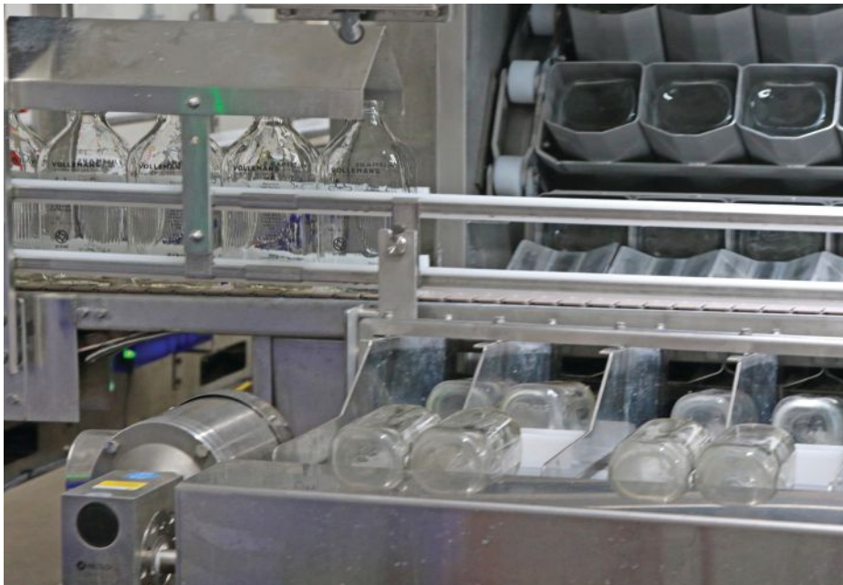
The glass bottles are returned to the plant, washed and sanitized before moving on a conveyor belt into the bottling area to be refilled.
