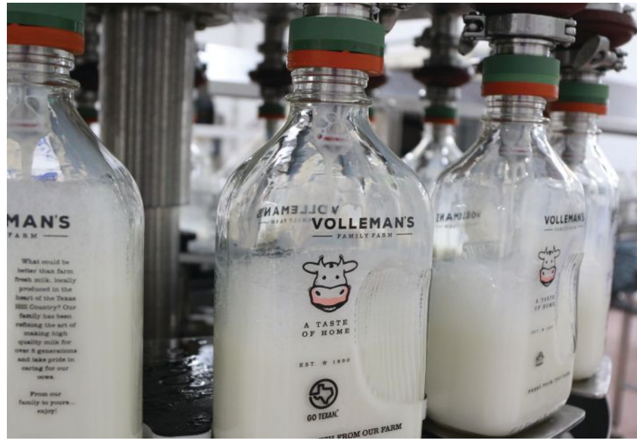
The bottles are filled by an entirely automated process before being crated and kept in cold storage until they're loaded on trucks for delivery.
