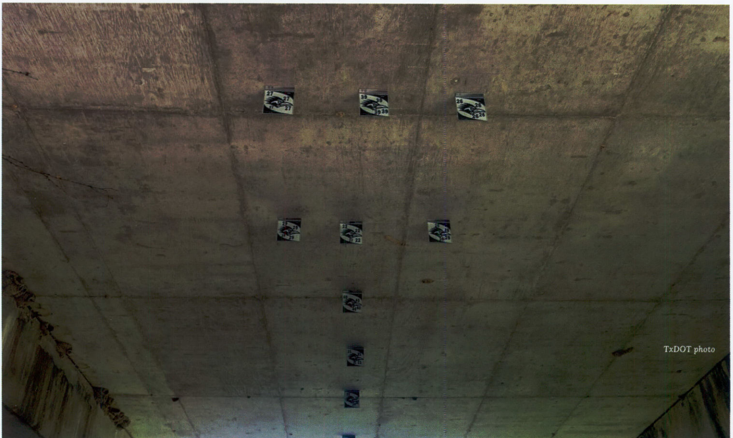
The system tracks the 3D spatial movement of targets placed on the surface of a bridge.
