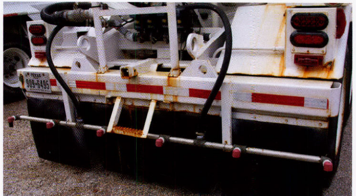
A third rear mud flap keeps brine away from the undercarriage of the tanker.
