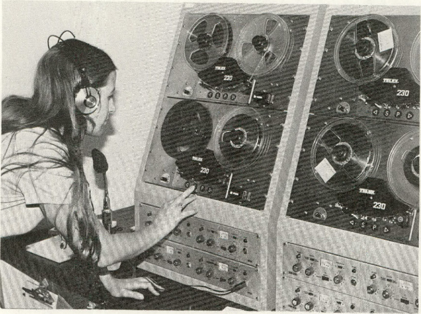
Two kinds of tape duplication are underway at the State Library. On the left cassette tapes are being duplicated for circulation. To the right the operator is converting open-reel tape to cassette tape.
