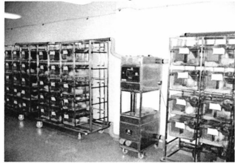
Fig. 8. HEPA-Filtered Ventilated Racks for Animal Housing
